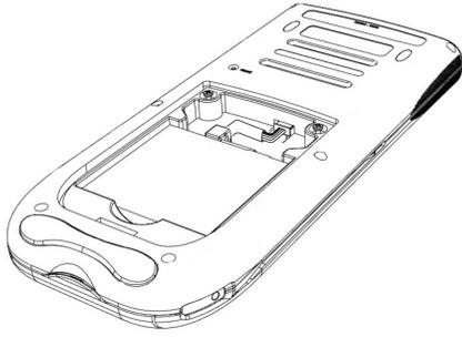
6. Replace the back panel and fasten the screws with a screwdriver.
