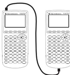
1. Firmly insert either end of the I/O unit-to-unit cable into the port.
