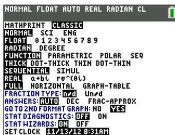
2. Press **[Y=]**. Turn off all functions and stat plots. Enter the **Y=** function to describe the fine. Use the **TEST** menu operations to define the piecewise function. Set the graph style for **Y1** to '·' (Dot-Thick).
