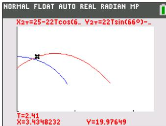
You can use  $\boxed{\text{TRACE}}$  to, in effect, take snapshots in time and explore the relative behavior of two objects in motion.
