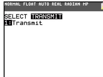
14. On the sending unit, press **1** to select **1:Transmit** and begin transmission. The receiving unit displays the message **Receiving...** When the items are transmitted, both units display the name and type of each transmitted variable.
