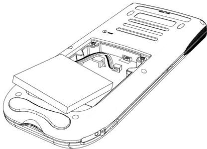
5. Thread the wire into the case to secure it. Insert the rechargeable battery into its compartment.
