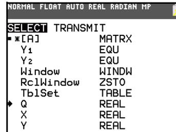
13. On the sending unit, press **►** to display the **TRANSMIT** menu.
