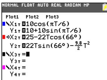
**Note:** Try setting the graph styles to  $\odot$  **X1T** and  $\odot$  **X2T**, which simulates a chair on the ferris wheel and the ball flying through the air when you press **GRAPH**.
